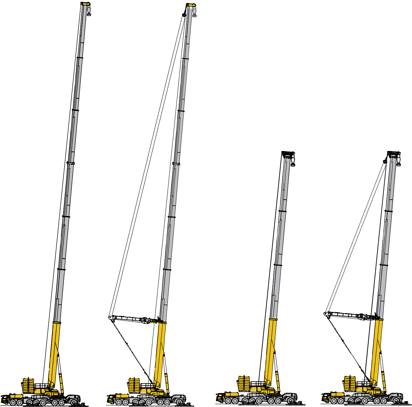
超起+四节主臂 Super lifting device + 4 boom sections
